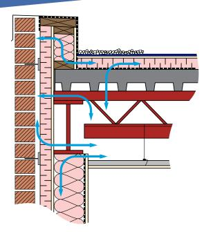
Arrows indicate air infiltration and exfiltration of the building.
